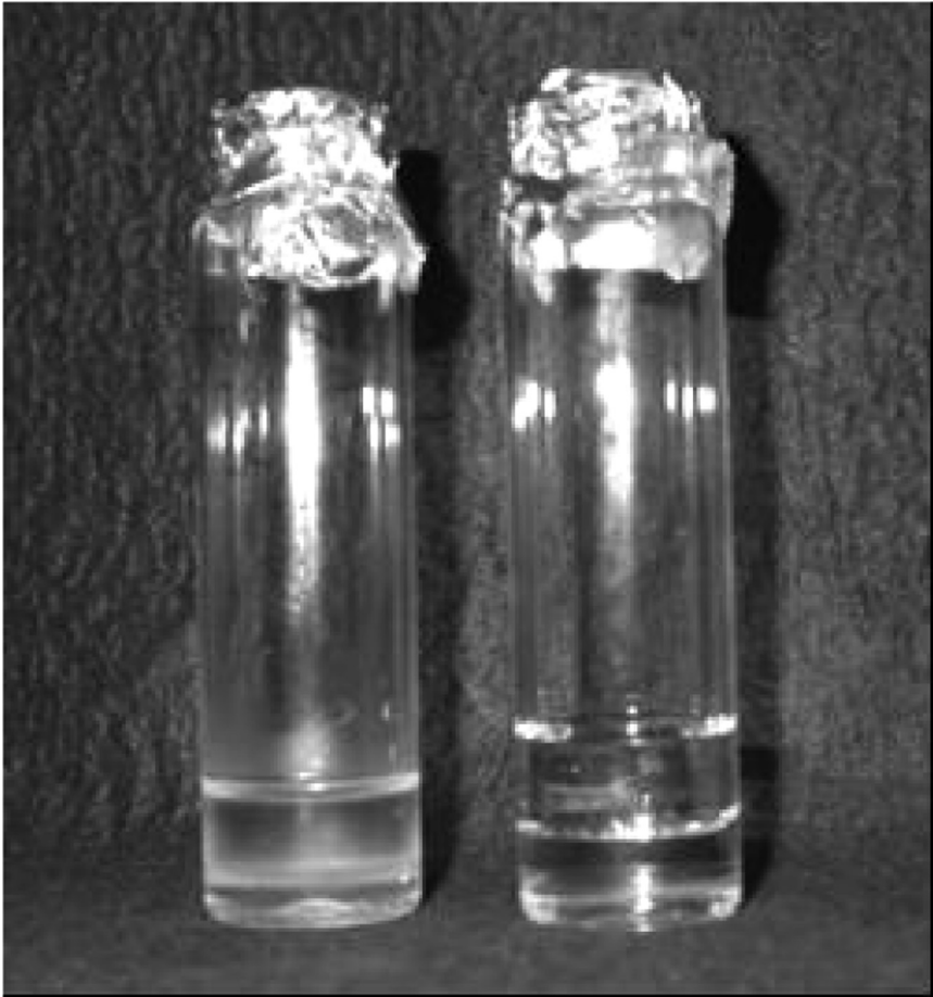
FIGURE 5 Left: Frekote 1711-1/DMSO. Right: Frekote 1711-1/water. A precipitate has formed at the interface of DMSO and Frekote. Much of the DMSO/heptane solution has absorbed into the Frekote phase.
